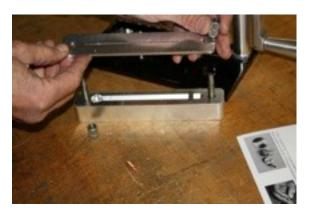
4) Remove the cover of the coil holder, be careful not to lose the springs under the cover.
